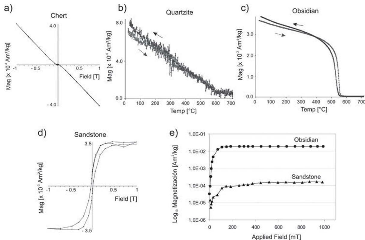
**Figure 4.** Representative examples of different rock-magnetic experiments carried out on the pre-burning material. (a and d) Hysteresis cycles. (b and c) Thermomagnetic curves and (e) Progressive IRM acquisition curves. Intensity values for each lithology are indicated.
