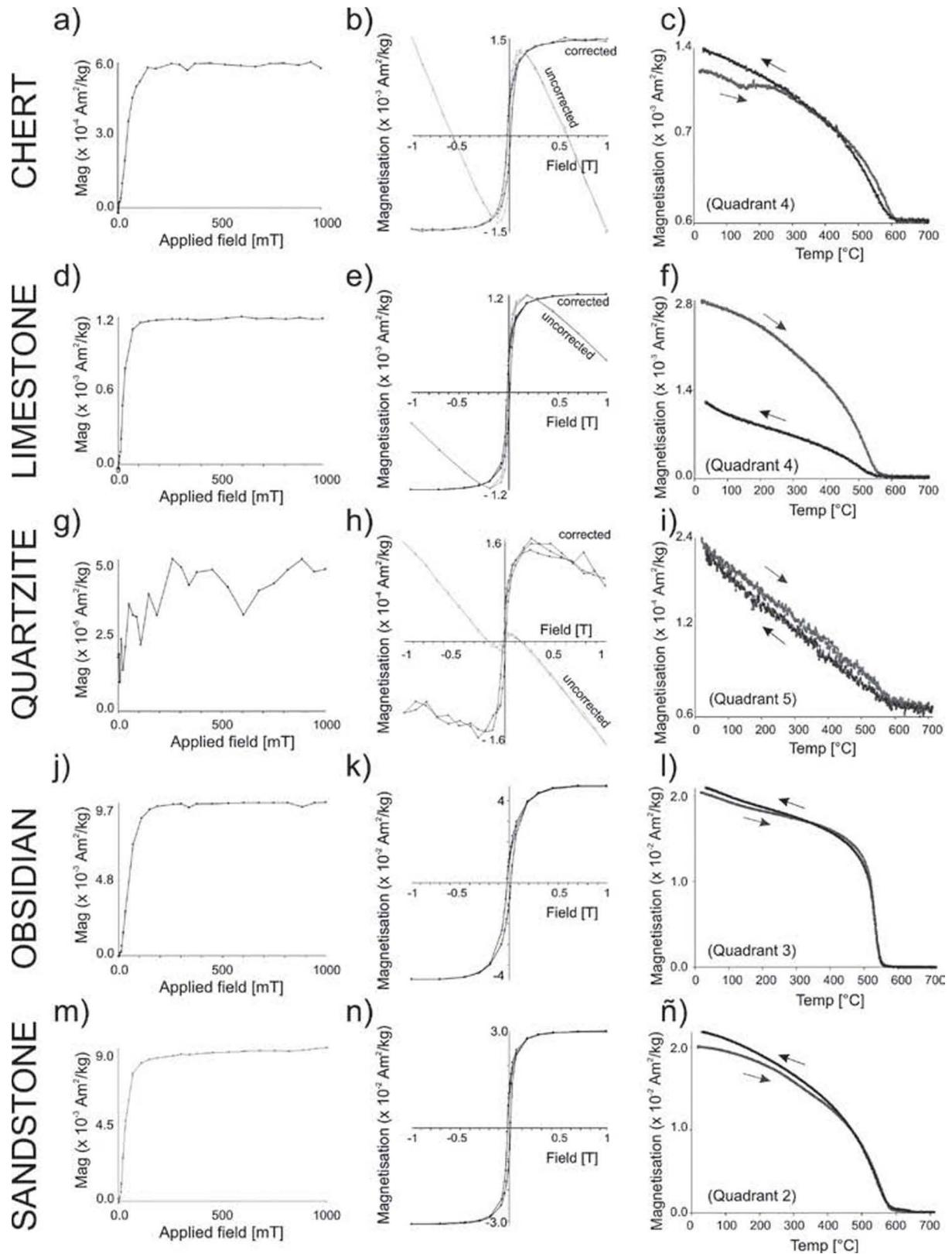
**Figure 7.** (a-ñ) Representative examples of IRM acquisition curves (left column), hysteresis cycles (central column) and their respective thermomagnetic curves (right column) for representative samples of each lithology after burning. Lithologies, applied field, intensity values and corresponding quadrant are indicated.
