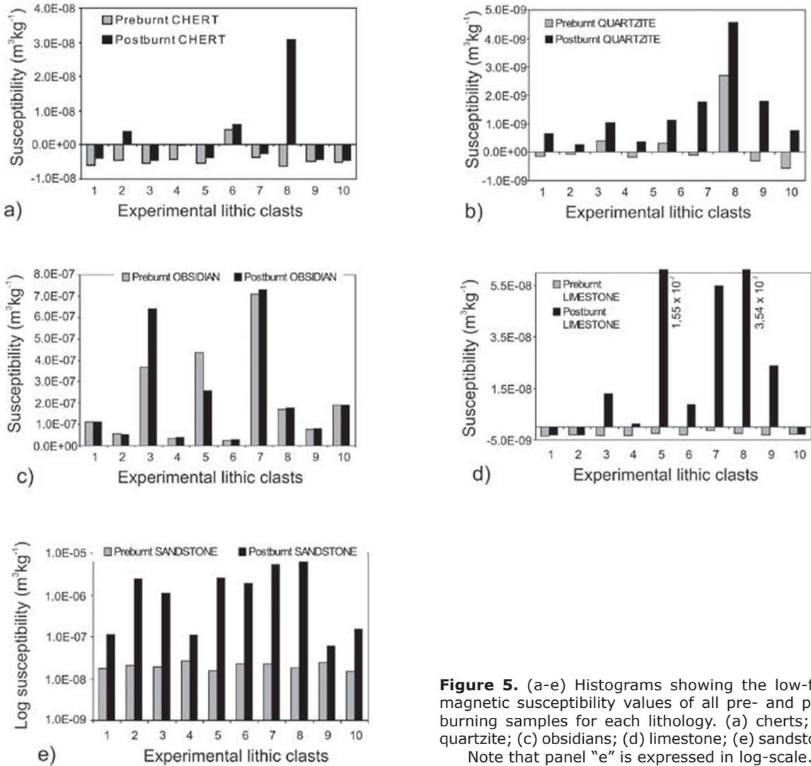
**Figure 5.** (a-e) Histograms showing the low-field magnetic susceptibility values of all pre- and post-burning samples for each lithology. (a) cherts; (b) quartzite; (c) obsidians; (d) limestone; (e) sandstone. Note that panel "e" is expressed in log-scale.
