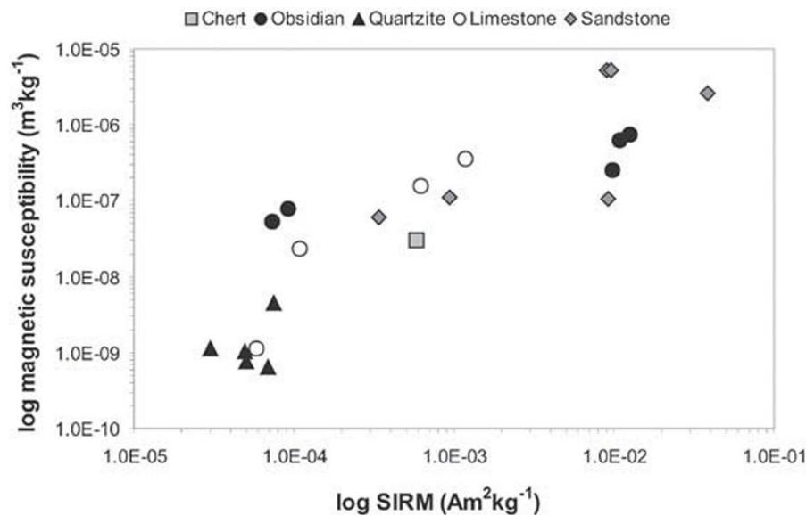
**Figure 9.** Scattergram of mass magnetic susceptibility vs. SIRM (Saturation isothermal remanent magnetisation) for the different post-burning lithologies. Diamagnetic values (five cherts and one limestone) are excluded.
