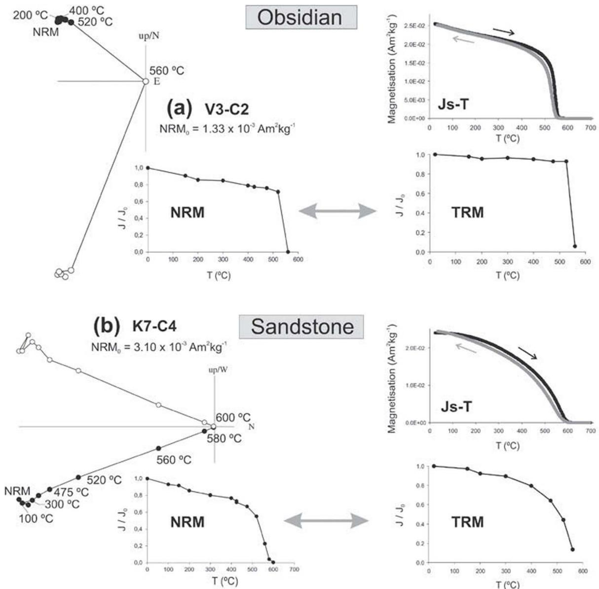
**Figure 10.** Thermal demagnetisation of NRM created during the artificial burning in the field and laboratory created full TRM for Obsidian (a) and Sandstone (b) samples. Also shown are corresponding continuous thermomagnetic (Js-T) curves. Please note that not exactly same samples were used for NRM and TRM demagnetisation experiments.
