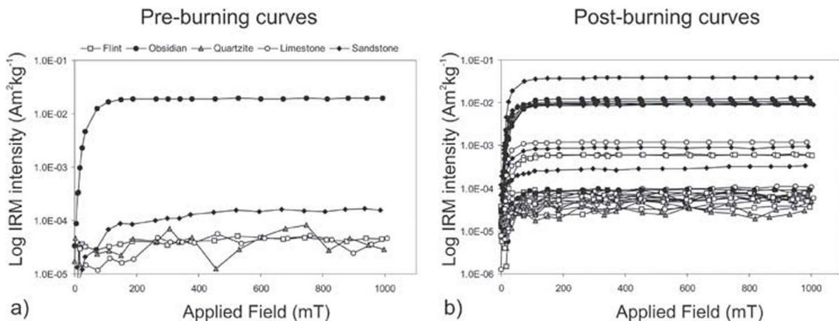
**Figure 6.** (a-b) Progressive isothermal remanent acquisition (IRM) curves before and after burning, respectively. Lithologies are represented in both graphs according to the legend shown in Figure 6a.
