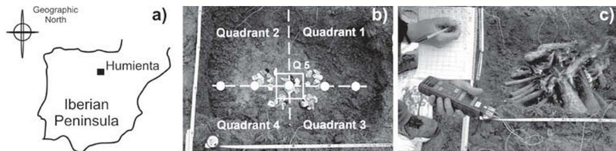
**Figure 1.** (a) Location of the site where the experiment was carried out. (b) Distribution of pieces by quadrants on the ground surface (Q5 refers to quadrant 5). White circles represent the location of thermocouples (T1-T5) at 0-1 cm of depth. Temperatures of the embers where the lithic pieces were located were recorded with T7 in Q5. (c) Temperature reading during the experiment.
