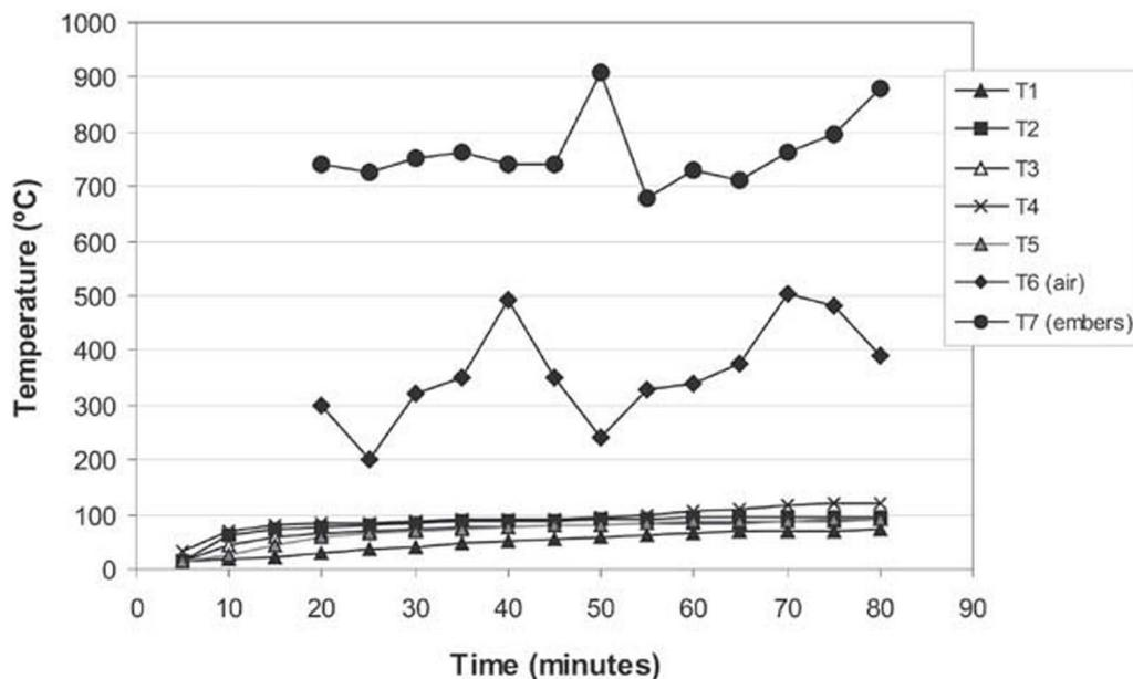
**Figure 2.** Temperatures recorded by each thermocouple during the experiment. T6 (temperature of the air) and T7 (temperature of the embers where the clasts were located). See text (field experiment section). Note that some temperature variations (e.g.: between min 45 and 60; T7) might correspond to wind variations or alternatively to some fuel addition during burning. More fuel help to increase the temperatures.
