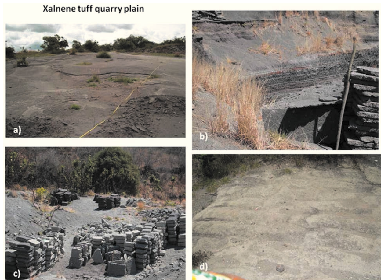
Figure 5. Views of the Xalnene tuff. (a) View of the quarry zone investigated by the resistivity soundings. (b, c) Views of the quarry operations, showing the trenches and the slabs cut from the ash layers. (d) View of marks left from quarry operations, modified by erosion. (a) View of marks produced by the mechanical excavator, partly eroded. The incision pattern with parallel groves can be observed.
