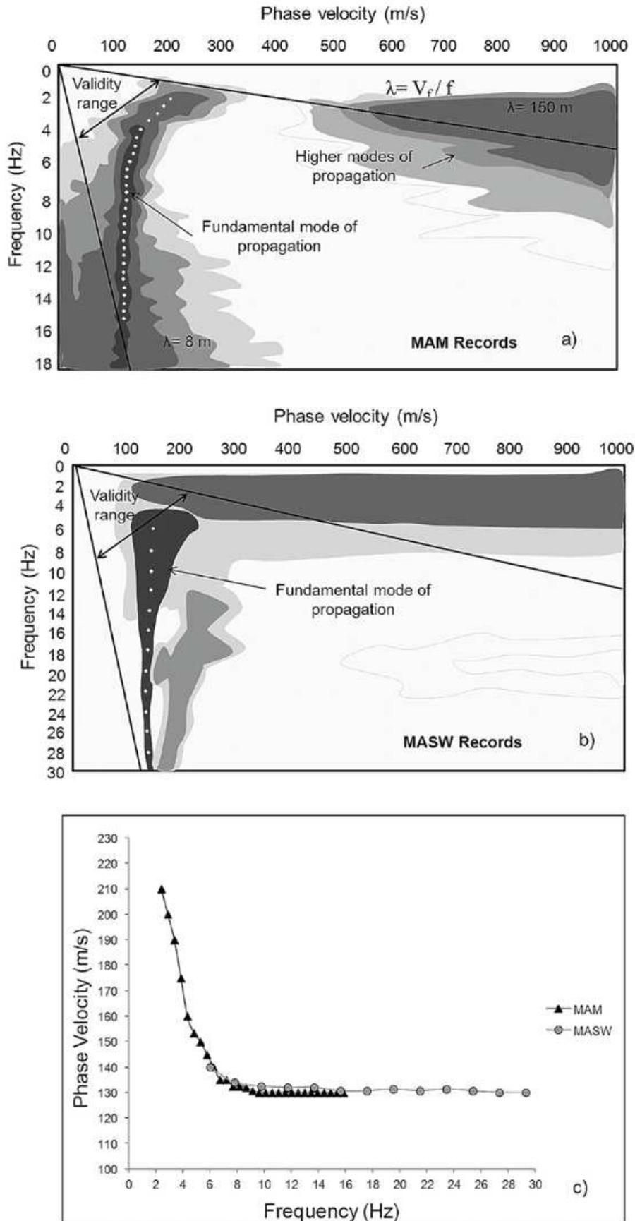
**Figure 7.** (a) The phase velocity-frequency image of MAM records. (b) The phase velocity-frequency image of MASW records and (c) Dispersion curves for active MASW and for passive MAM corresponds to the line L5T1.
