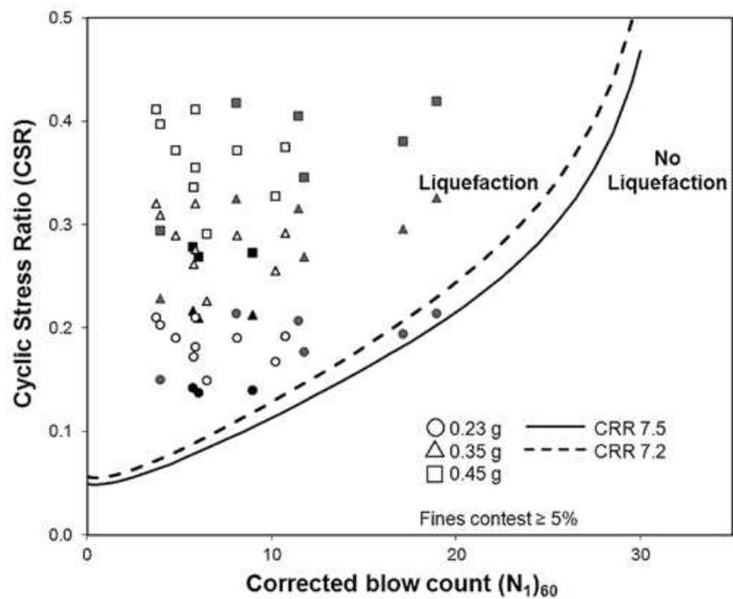
**Figure 11.** Curve for calculation of CRR versus  $(N_1)_{60}$
