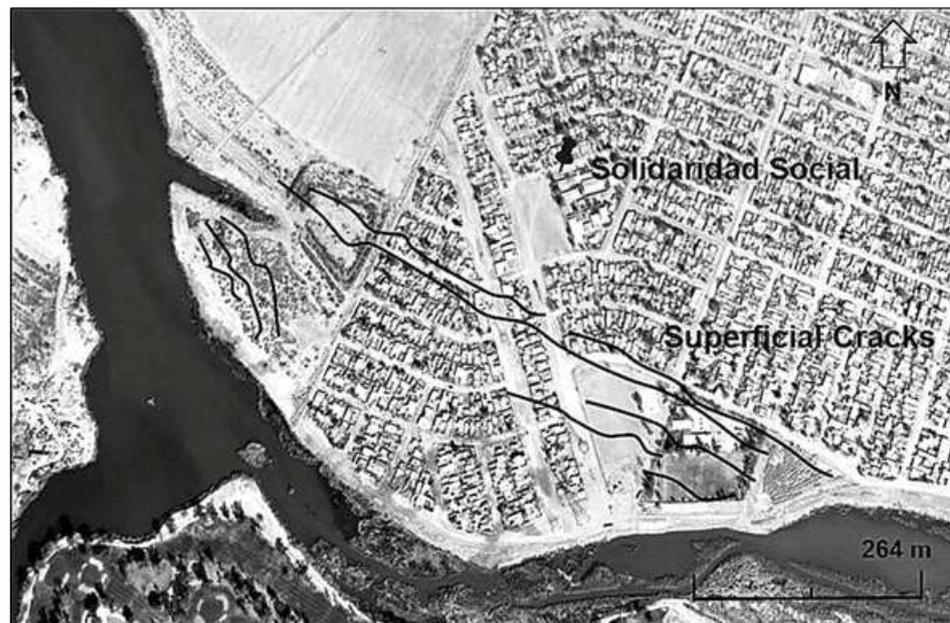
**Figure 2.** Superficial cracks and fractures.
