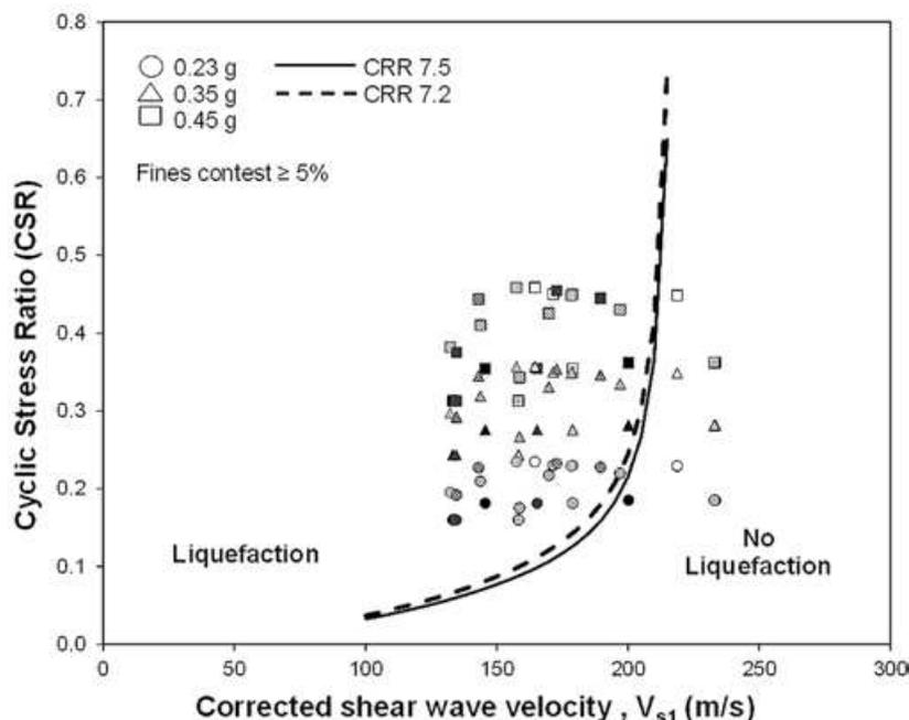
**Figure 12.** Curve for calculation CRR versus  $V_{s1}$
