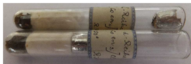
Figure 16 Two vials of PhD student Richard Hessen containing the [ \Delta -(d-)] and [ \Lambda -(l-)]dinitrobis(ethylenediamine)cobalt]Cl compounds obtained by conglomerate chiral resolution with S- and R-camphorsulfonate salts. Vials from the Alfred Werner collection of the University of Zurich.
