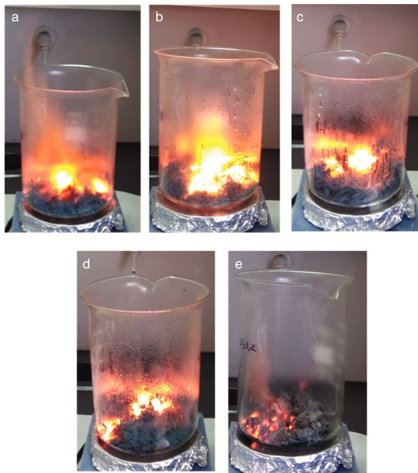
Fig. 1 – Digital images of the combustion reactions: (a) \text{CoCr}_2\text{O}_4 , (b) \text{Co}_{0.8}\text{Mg}_{0.2}\text{Cr}_2\text{O}_4 , (c) \text{Co}_{0.5}\text{Mg}_{0.5}\text{Cr}_2\text{O}_4 , (d) \text{Co}_{0.2}\text{Mg}_{0.8}\text{Cr}_2\text{O}_4 , (e) \text{MgCr}_2\text{O}_4 .
