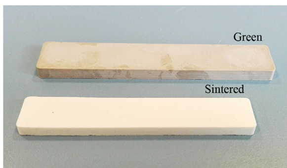
Fig. 12 – Green part (top) and sintered part at 1410 °C (bottom) of the optimal P3 porcelain feedstock processed by CIM.
