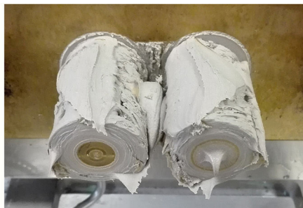
Fig. 5 – Appearance of feedstocks obtained after the mixing process for porcelain P2-48 vol.% (left) and porcelain P3-55 vol.% (right).
