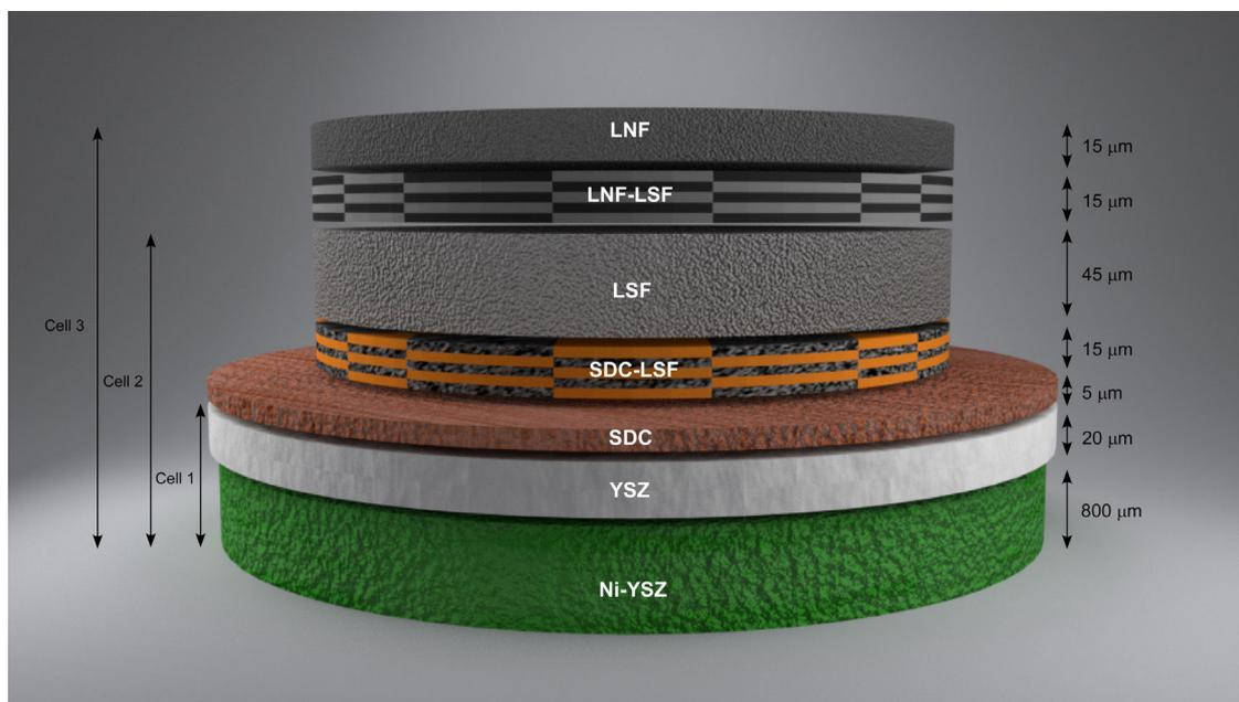
Fig. 1 – Scheme of the used layers in each cell.
