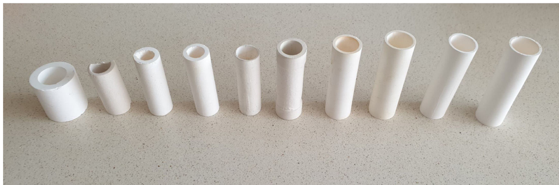
Fig. 1 – Picture of different ceramic passive samplers constructed, showing different dimensions.
