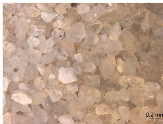
Fig. 1 – AG clay. Material retained in 200-mesh sieve. Quartz particles stand out for their typical vitreous luster.
