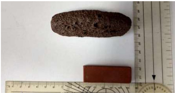
Fig. 4 – Rectangular body before and after firing at 1300 °C.
