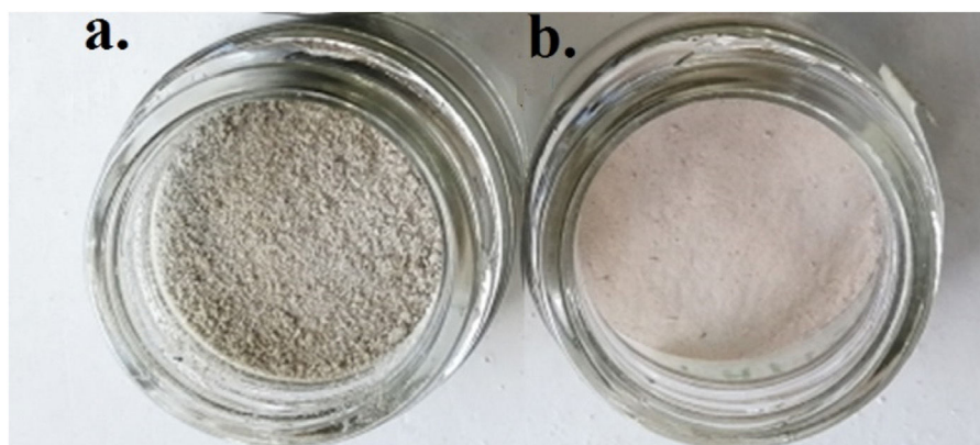
Fig. 8 – (a) FA after fusion with NaOH. (b) Synthesized FAU zeolite.
