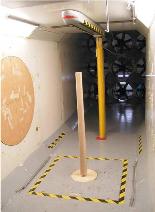
Figure 12. Cross-sectional wind test on pier 4.
