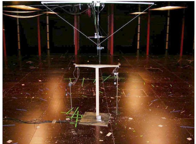
Figure 16. Scale model of a single pier for wind tunnel test.
