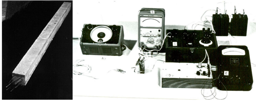
Figure 2. Left: prestressed beam manufactured for the work of the thesis. Right: set of equipments to measure the electrical resistance due to the concrete itself, multimeter for measuring the corrosion potential and in the right-down corner the galvanostat (white cover in the figure) and the black multimeter to measure the current.
