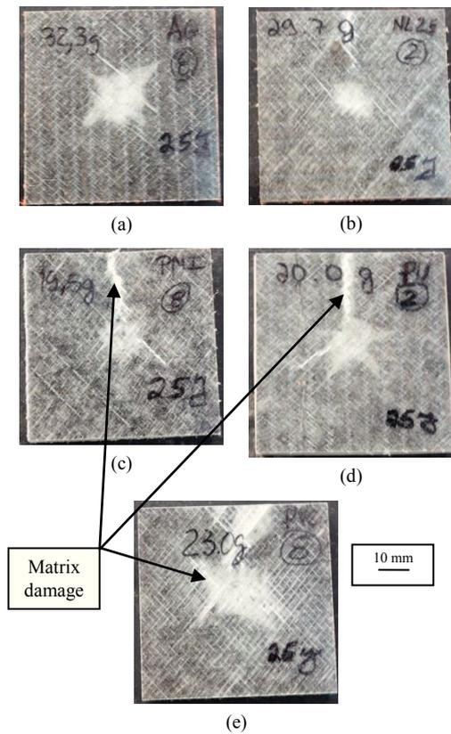
Fig. 8. Specimens impacted at 25 J: (a) standard cork agglomerate (AG), (b) NL25, (c) PMI, (d) PUR and (e) modified PVC. Cork based specimens clearly show less damage than other sandwich specimens.
