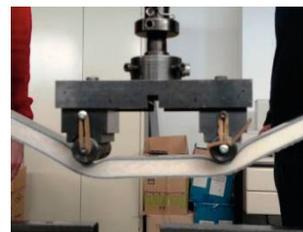
Fig. 5. Sandwich specimen with PUR foam core during four-point bending testing.
