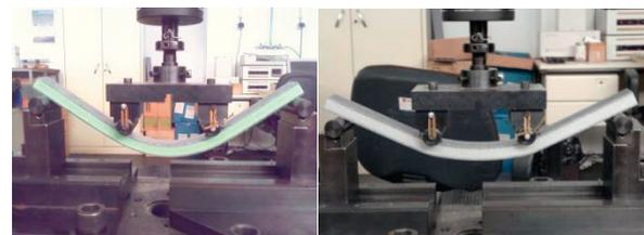
Fig. 4. Sandwich specimens during four-point bending testing: modified PVC foam (left) and PMI foam (right) cores.
