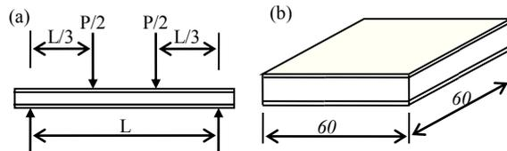
Fig. 1. (a) Third-point loading configuration for four-point bending tests, according to ASTM C 393-00, and (b) low velocity impact specimens.
