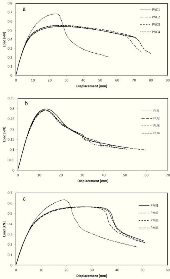
Fig. 2. Load-deflection curves from four-point bending tests for sandwich structures with polymer foam-based core materials: (a) Airex® C 70.75 modified PVC foam, (b) PUR foam, and (c) Rohacell® PMI foam.
