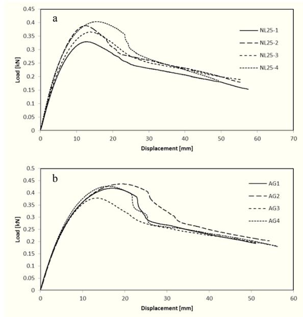
Fig. 3. Load-deflection curves from four-point bending tests for sandwich structures with cork-based core materials: (a) NL25 cork agglomerate and (b) standard cork agglomerate.
