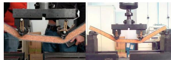
Fig. 6. Cork core-based sandwich specimens during four-point bending testing: NL25 (left) and standard cork (right) cores.
