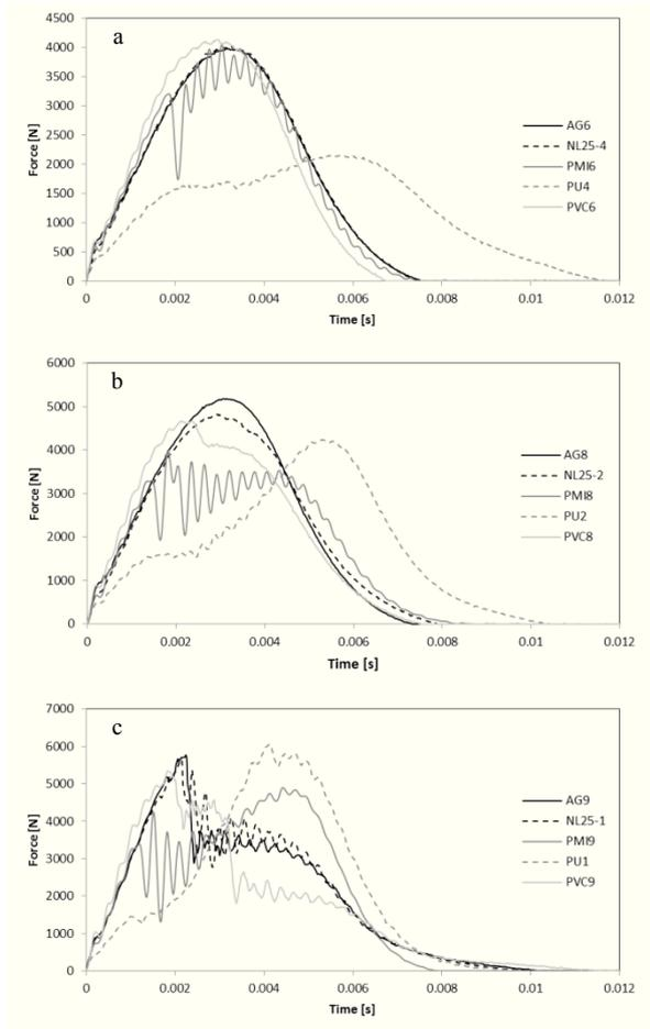
Fig. 7. Force-time plot histories of sandwich specimens subjected to low velocity impact: (a) 15 J, (b) 25 J, and (c) 40 J energy levels.
