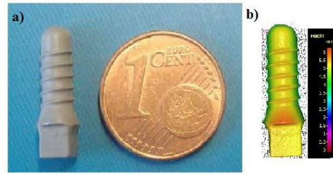
Fig. 7. "Green" implant a) in real scale and b) analyzed by IFM.
