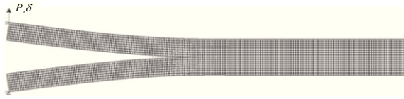
Fig. 4. Mesh and boundary conditions used in the numerical simulation of the DCB test.
