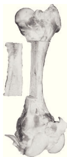
Fig. 1. Bovine femur – detachment of a slice of cortical bone tissue in the diaphysis region.
