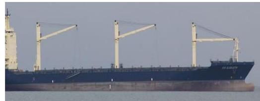
Fig. 1 Container ship with the 3 cranes and its pedestals.
