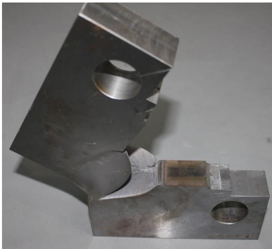
Fig. 11. Flat surface specimen after testing, revealing typical plane stress behaviour.
