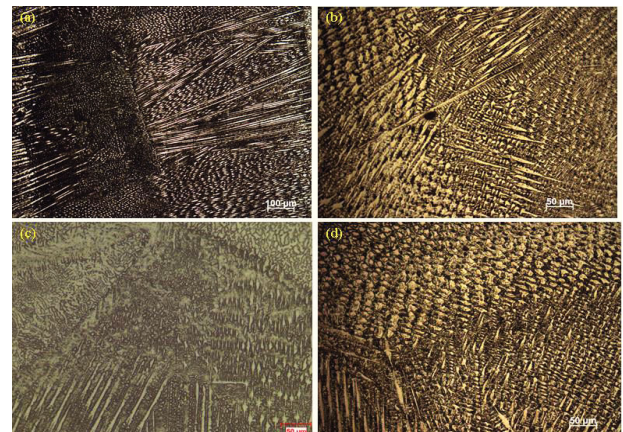
Fig. 5. Weld microstructure showing the multi-directional grain growth in CCGTA weldments employing (a) ER2553 (b) ERNiCrMo-4 and PCGTA weldments employing (c) ER2553 (d) ERNiCrMo-4 fillers respectively.
