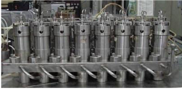
Fig. 1. Sixteen stage centrifugal extractor bank assembly.
