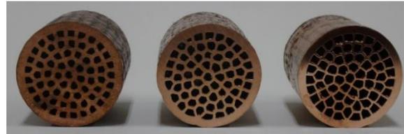
Fig. 1. UniPore samples with different porosities ( $p = 0.32, 0.49, 0.58$ ).
