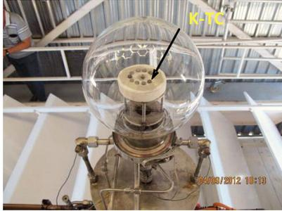
Fig. 2. Reaction chamber used for nitriding tests.
