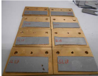
Fig.1. Test sample of HSLA 380 for friction test on pin-on-disc machine.
