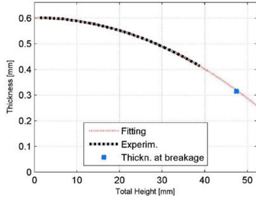
Fig. 3. Results from adjusting parameters from Eq. 15, for DP590.
