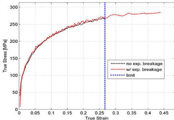
Fig. 5. Biaxial stress-strain determination for AA5754, using experimental strain data and proposed fitting equation.
