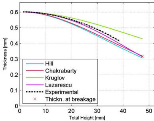
Fig. 2. Comparison of methodologies for determining the thickness for DP590.
