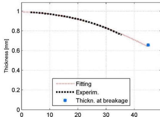
Fig. 4. Fitting equation for thickness evolution using proposed methodology, for AA5754.
