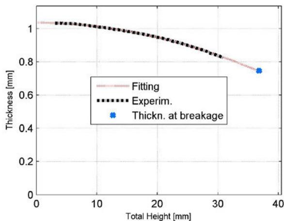
Fig. 6. Fitting equation for thickness evolution using proposed methodology, for AA6061.
