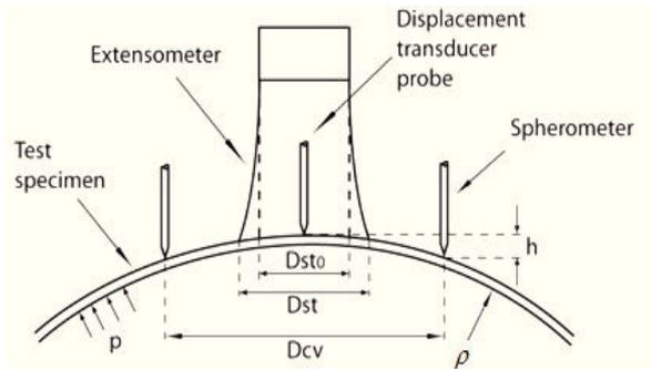
Fig. 1. Variables used for evaluation of stress and strain.
