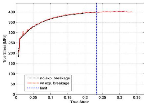
Fig. 7. Biaxial stress-strain determination for AA6061, using experimental strain data and proposed fitting equation.
