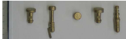
Fig. 1. Microscrews produced by \mu PIM.
