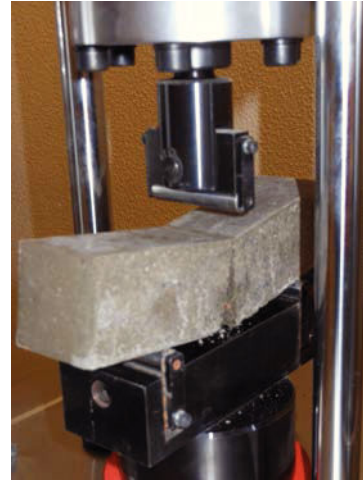
Fig. 2. Testing set-up for three-point bending.
