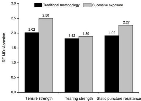
Fig. 3. Comparison of the reduction factors ( RF_{MD+ABR} ) obtained by the traditional methodology and by the successive exposure to both degradation agents.
