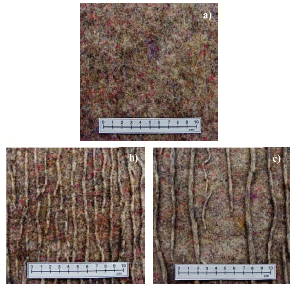
Fig. 1. Nonwoven geotextile: a) after mechanical damage (global appearance similar to undamaged – the defects cannot be seen at this magnification), b) after abrasion and c) after mechanical damage followed by abrasion.
