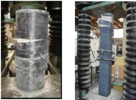
Fig. 2. Failure of CFRP confined specimens.
