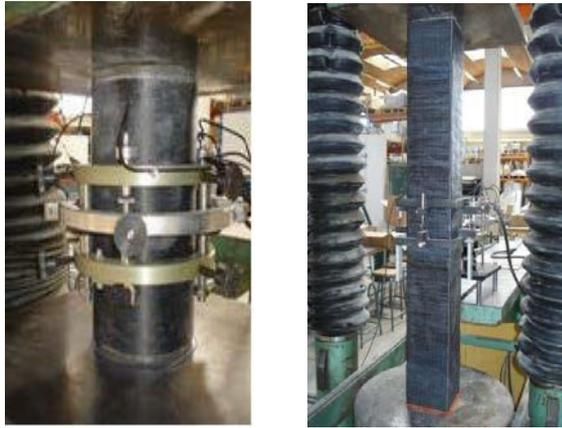
Fig. 1. Test set-ups for circular and square columns.
