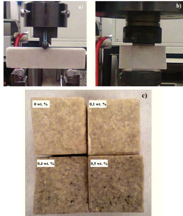
Fig. 2. a) Flexural, b) Compressive testing set-ups and c) Fracture surfaces of PM test specimens after flexural tests
