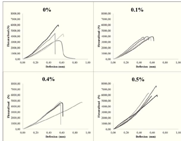
Fig. 3. Flexural load-deflection curves.
