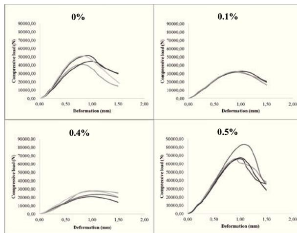
Fig. 4. Compressive load-deflection curves.
