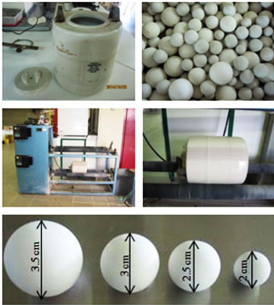
Fig. 1. Wet milling machine and the balls' dimensions used.
