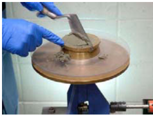
Fig. 5. Flow-table test procedure.
