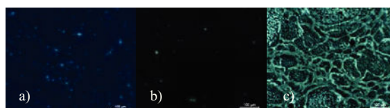
Fig. 6. Fluorescence micrographs of: a) recycled HDPE modified binder, b) binder recovered after modification, and c) polymer recovered after modification.
