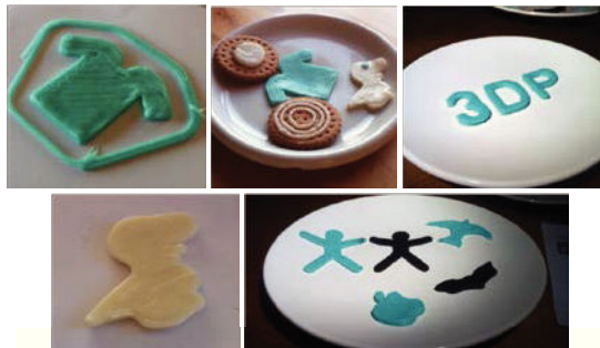
Fig. 4. 3D printed shapes with sugar paste.
