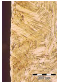
Fig. 6. Surface of the TiAl casting before chemical milling, without traditional alpha case.
