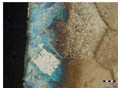
Fig. 1. Ti10V2Fe3Al alloy microstructure, alpha case on sample's surface (left layer), etched with Kroll's reagent [5].
