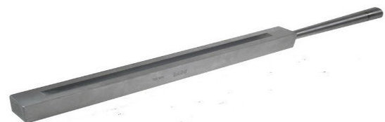
Fig. 1. Metallic strip ingot mould used.
