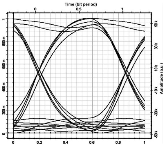
Figure 5. Eye diagrams of the bipolar encoding structure.
