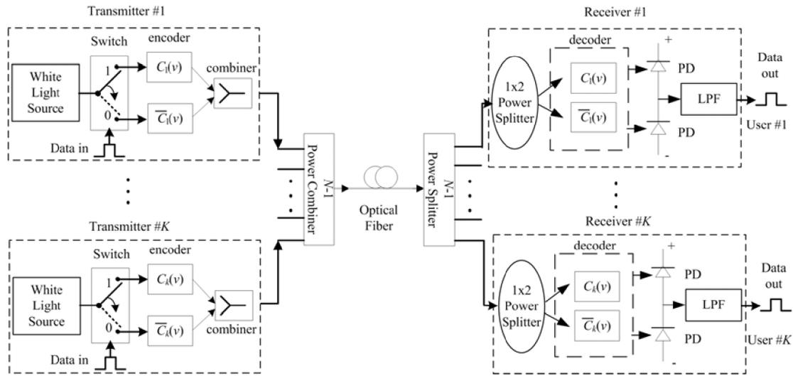
Figure 1. The system configuration of the SAC-OCDMA system.
