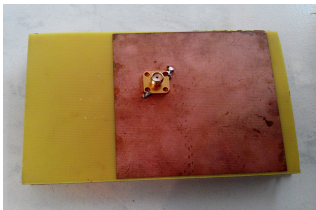
Fig. 14. Fabricated structure of ground.
