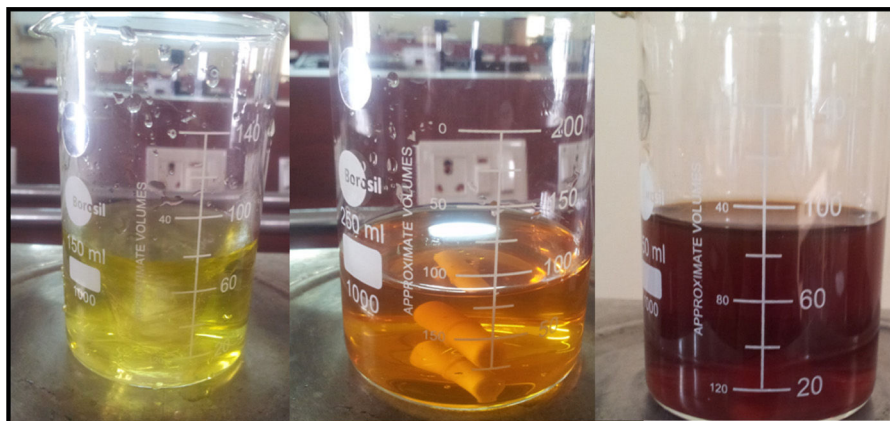
Figure 1. Increase in the color intensity of the reaction mixture with time for 5, 30 and 60 min.
