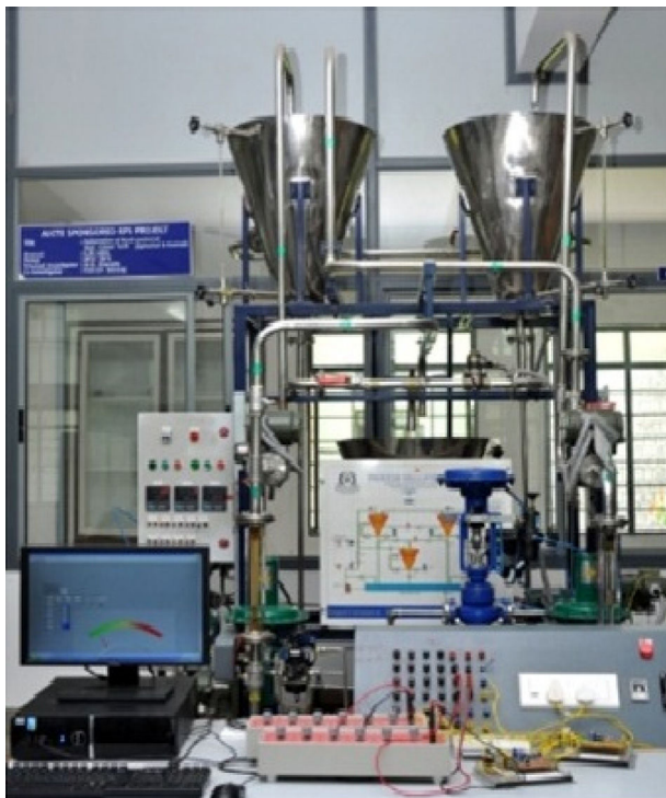
Fig. 15. Conical tank experimental setup.
