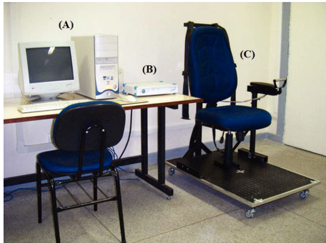
Figure 1 - System acquisition: (A) PC, (B) System acquisition and signal conditioning model SPIDER 8 and (C) Strength Measuring Station (SMS).
