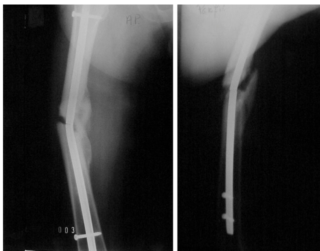
Figure 3 and 4 - A fractured femoral nail in an unhealed femoral fracture (Anterior-Posterior and lateral radiographs)
