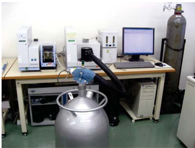
Figure 8. Nitrogen-based cooling system used in the test.
