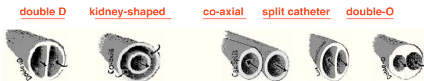
Figure 4 Catheters classified according to their lumen section.
