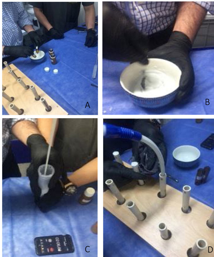
Figure 2 Cementation procedure. A. Mixing. B. Homogenisation. C. Packing in the syringe. D. Placing in the PVC tubes.
