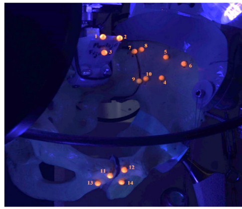
Figure 4 Markers fixed to each bone segment and prepared for monitoring. The illumination with ultraviolet light can be seen. Sacroiliac joint: 7–8 = upper pair, 9–10 = lower pair. Symphysis: 11–12 = upper pair, 13–14 = lower pair. Markers 1, 2, 3 and 4, 5, 6 define auxiliary coordinate systems fixed to the sacrum and the fractured blade, respectively.
