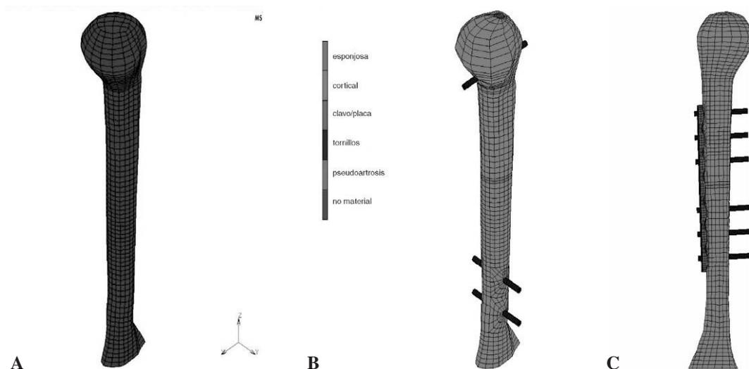
**Figure 3.** Grid models of a healthy humerus (A), humerus with nailing (B) and humerus with plate (C). Performed using MSC-PATRAN® (IBM, Armonk, USA).
