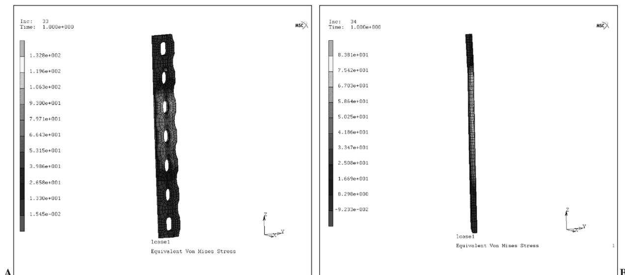
Figure 5. View of weight-bearing distribution during torsion. Tension is indicated in megapascals.
