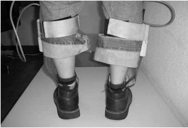
Figure 3. System of instrumented insoles adapted to the subjects footwear.
