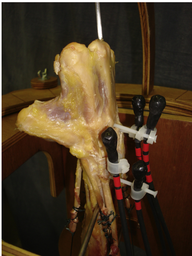
Figure 1 Image of the final aspect of one of the anatomical specimens placed on the support designed for this study. The sensors were placed on the radius, scaphoid, triquetrum and capitate bones.
