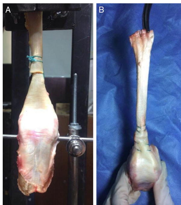
Figure 1 Repair techniques. (A) Dresden repair. (B) Kessler repair.
