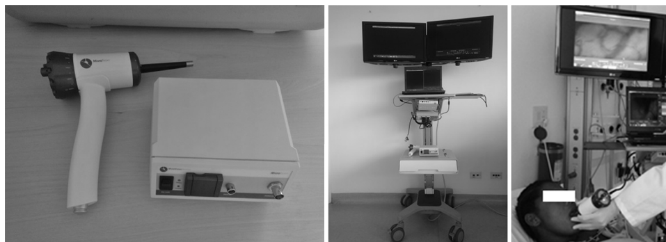
Fig. 1 – Sidestream dark-field (SDF) system: system for use as a hand microscope in the study of microcirculation at the patient's bedside in real time. Consists of a guide-light surrounded by green light emitting diodes (530 nm) that penetrate the tissue, illuminating the microcirculation. The green light is absorbed by the hemoglobin of the red blood cells, and a magnifying glass projects the image on a video camera (Reproduced with permission from Dr. Gustavo Adolfo Ospina Tascón).
