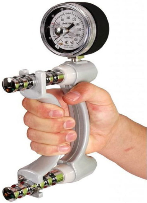
Figure 1 Jamar dynamometer. Isometric Hand Grip Strength is a simple, non-invasive, inexpensive test used as a predictor of adverse health outcomes that can be measured using a variety of digital, analog, hydraulic, and Smedley-type dynamometers.
