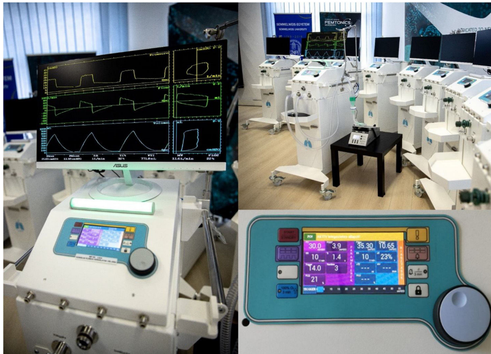
Fig. 1. Luca mechanical ventilator with close-up of the user interface (online version: colour; print version: black and white).
